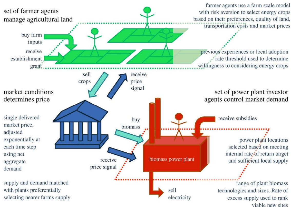
Figure 1: Schematic of the main agent processes and interactions within the perennial energy crop market model
