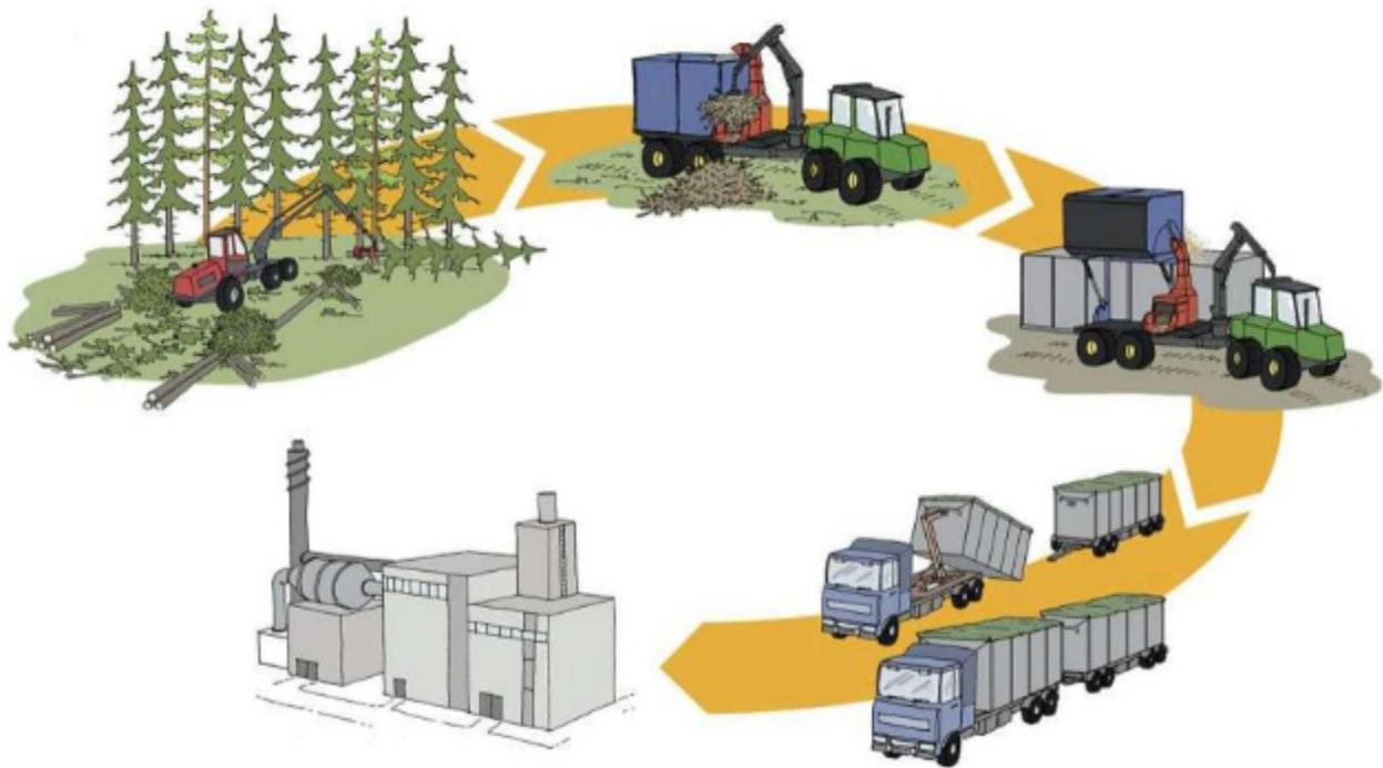
**Figure 1** Wood chipping process (LUT 2013)
